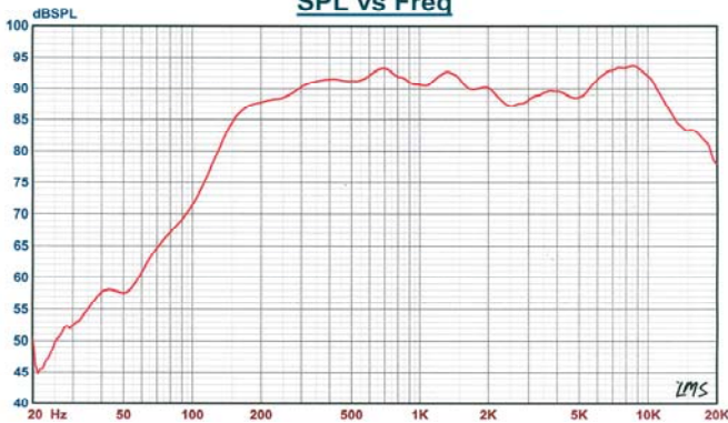
Sound pressure levels at 1W/1m w/P-4x6 SPL vs Freq
